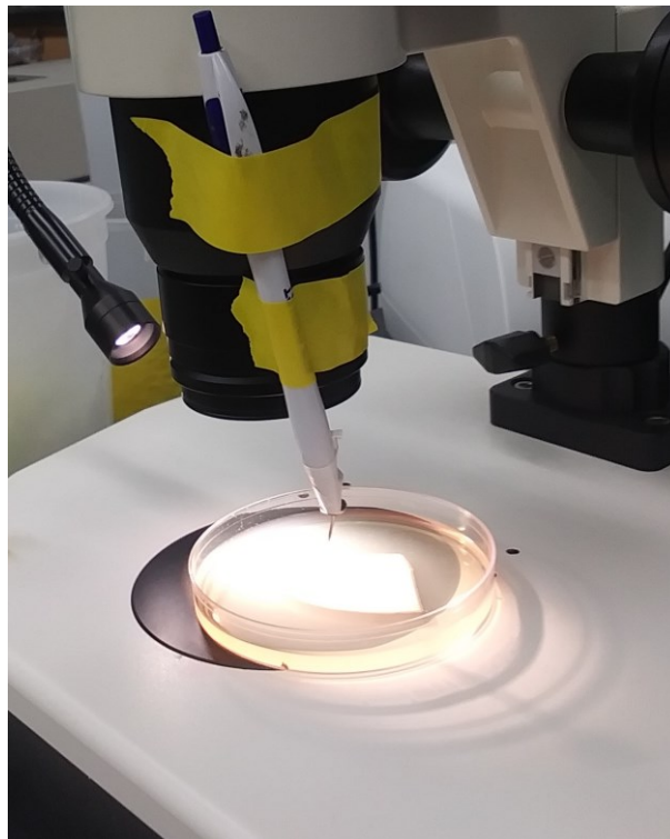
Figure 10. Colony picking by a flame sterilized pin. The coarse adjustment knob of the dissecting microscope is used for the precise up-down movement of the colony picking pin.
