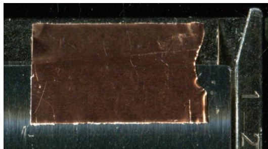
Figure 7. Example for placement of a copper tape. The copper tape does not reach above the upper edge boundary of the MALDI adapter.
